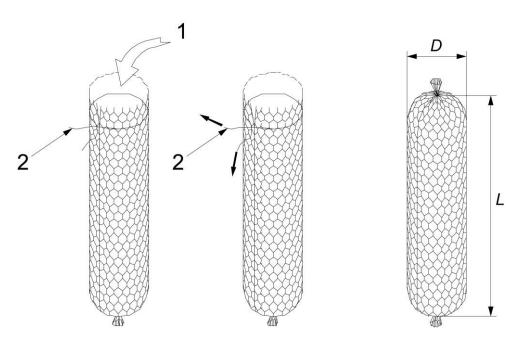
Key: 1 filling; 2 lacing wire; D diameter; L length
