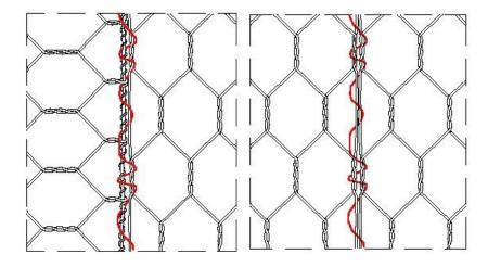
Figure 4 – Example of connection using lacing wire
