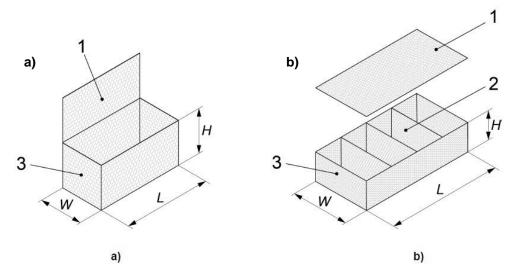
Key: 1 lid; 2 diaphragms; 3 end panels; H height; L length; W width
