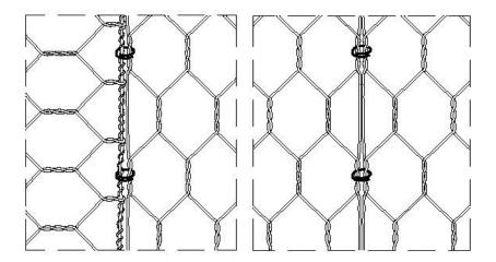
Figure 5 – Example of connection using C-rings
