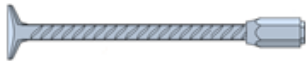
Figure A.1.3: Example for type 3 - stud connector of a combination of type 1 and type 2
